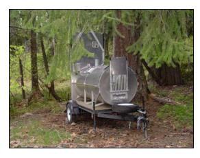
Here is a more recently developed culvert trap (explained in detail below). Notice the trap is placed in a shady trap site, on level ground, and is fully secured using all 4 stabilizers and wheel chocks.
