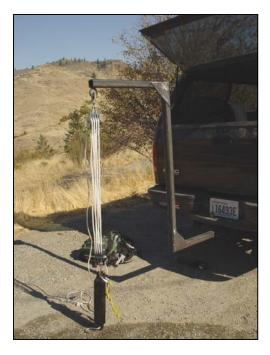
Here is a simple device that can be used to weigh bears captured in culverts. The pulley system cuts the weight by 75% and a single person can easily lift a 300-pound bear.
