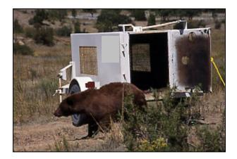
Here is another good culvert trap design. It has a side-mounted door (notice the rope attached to the door for safe release from a vehicle), and small grates for avoiding broken teeth and claws.
